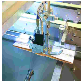
Fully integrated adhesive system complete with glue-line inspection system.
