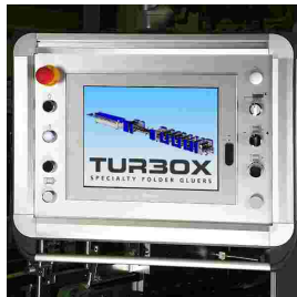
BOXFLOW® CONTROL – intuitive touch screen monitors for machine operation.
