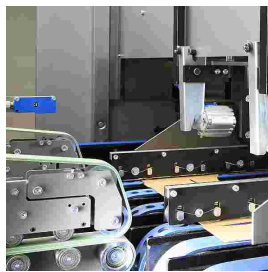
Precise transfer of blanks from the servo-driven ACE-Feeder to the next unit.
