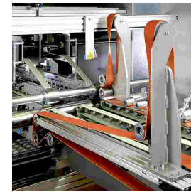
Movable top folding belts for specialty folding boxes.
